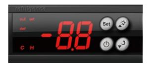
The control panel is located on the back, interior wall, in the upper right-hand corner. Under normal operation, the LED display shows the internal temperature of the cabinet. If you have any other questions regarding the operation of this unit, please call our Customer Service Department at **1-800-932-4267** (9:00AM to 5:00PM ET).
