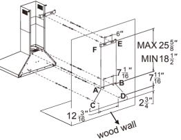
Screw the chimney mounting parts into Ø 8mm sized wall plugs on E,F points which are provided with your product.
