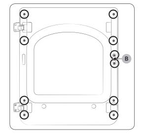
**3.** Remove the two screws from the lever holder, and then remove the holder cover.
