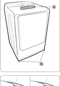
Using a level (A), check if the dryer is level side to side and then front to back. If the dryer is not level, adjust the leveling feet (B) at the bottom of the dryer. Then, check if the dryer is level again.
