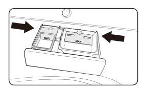
**2.** Push the ends of each side of the case at the same time. When you feel the ends push, pull out the dispenser drawer.
