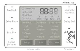
Self Clean is a self-cleaning cycle that removes mold that may occur inside the washer.
