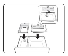
**3.** Remove the inserts from the 3 compartments. Rinse the inserts and the drawer with warm water to remove traces of accumulated laundry products.
