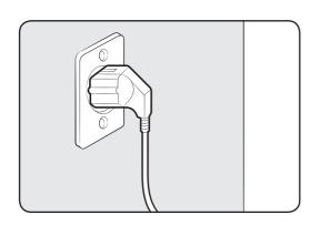
Plug the power cord into a 3-prong, well grounded 120 volt 60 Hz approved electrical outlet protected by a 15-amp fuse or comparable circuit breaker.
