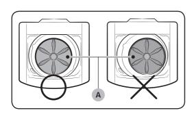
See if the washer is level by checking the position of the tub:
