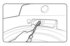
**4.** To clean the drawer opening, use a small, non-metal brush to clean the recess. Remove all residue from the upper and lower parts of the recess.
