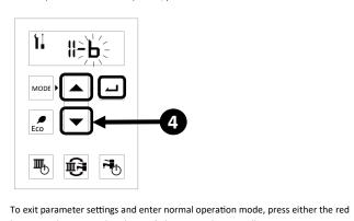
button on the PC Board or the Mode button on the controller.
