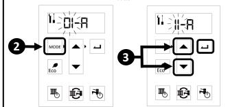
Press the (Up) or (Down) arrows to change the selection for the setting number (such as 11-A or 11-b). Then, press the **Select** button.
