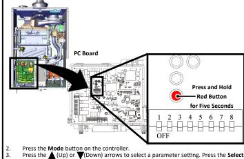
Press the (Up) or (Down) arrows to select a parameter setting. Press the **Select**
