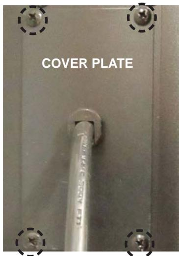
**A.** Remove the cover plate from the left side of the appliance by removing the four screws, as shown above.
