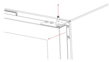
Remove the hinge bushing from the adaptor plate. A new bushing is included in the literature pack with your unit.
