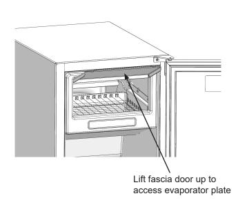
Refer to your cleaning solution instructions to determine the proper amount of cleaning solution to add based on 2 quarts (1.9 liters) of water. Lift fascia door up to access evaporator plate. Pour the cleaning solution slowly on the evaporator plate so it flows down into the fresh water reservoir.
