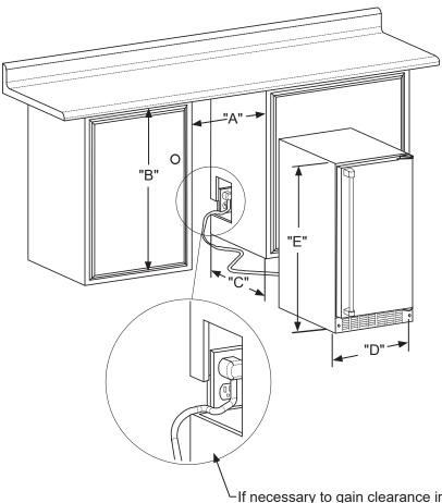
If necessary to gain clearance inside the roughin opening a hole can be cut through the adjacent cabinet and the power cord routed through this hole to a power outlet. Another way to increase the available opening depth is to recess the power outlet into the rear wall to gain the thickness of the power cord plug. Not all recessed outlet boxes will work for this application as they are too narrow, but a recessed outlet box equivalent to Arlington #DVFR1W is recommended for this application.
