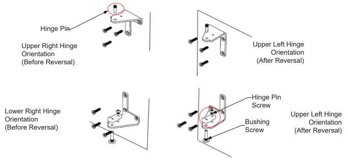
5. Using a 5/32" Hex Key, remove the Upper and Lower Hinge Brackets from the door, saving all components. Remove black plugs from opposite side of door. flip the Upper Hinge Bracket and reattach the Hinge Bushing and screw into place on the opposite side of the door (where plugs were removed). Remove the Cam Closer from the Lower-Hinge Bracket and attach it to the opposite side.
