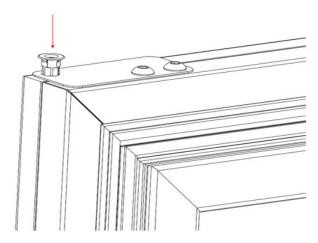
Align hinge bushing with top hinge and reinstall upper hinge pin using 1/8" Hex Key so that the pin is flush.
