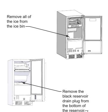
Replace the splash shield if removed. Turn the ice machine back on by pressing and holding the "ON/OFF" icon for 3 seconds. The display will indicate "ICE" mode. Press and hold the "MENU" icon until a flashing "CLEAN" is displayed. Press the "ON/OFF" icon until "CLEAN" stops flashing. Your ice machine will now enter the clean cycle.
