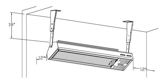
**IMPORTANT NOTE:** Use only the mounting brackets provided with this heater. Heater must be installed in a horizontal manner parallel with the ground. The heater can, however, be tilted upward to a maximum of 30 degrees. NEVER mount the heater on a vertical axis. Such an installation is considered unsafe and will void all warranties.
