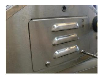
Remove screws from right end Access Cover
