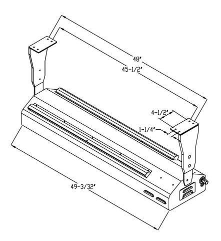
If it has been determined that the heater be mounted straight down, i.e., with no angle on its pivot point, then the heater should be mounted **NO CLOSER** than 14" from the ceiling. The side clearances should be **NO CLOSER** than 12" to a side wall, and the rear clearances should be **NO CLOSER** than 12" to a rear wall. Use the **LOWEST** pair of holes in the mounting bracket extension arms. See illustration below.
