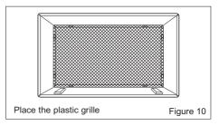
**3** Fasten the 4 washer screws to secure the grille to the wall sleeve. If you need plastic nuts to mount plastic grille to the inside of the wall sleeve, there are plastic nuts in the installation kit. The nuts are installed from the inside of the sleeve and are pressed into the square holes of the rear flanges.
