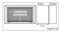
5 If the depth of your existing wall sleeve is less than or equal to 18", skip to step 7. Otherwise, cut the baffles and the support blocks according to Length A in the table below.
