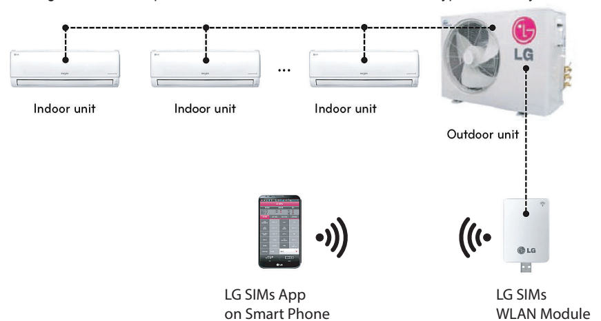
Figure 131: Example of a SIMS WLAN Module Used with a Typical DFS System.
