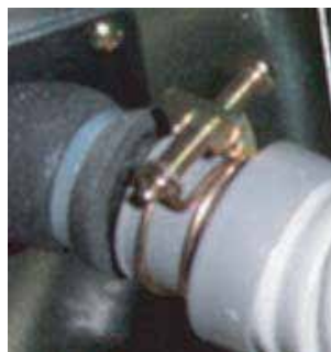
Clamp the Flexible Drain Hose Connection
