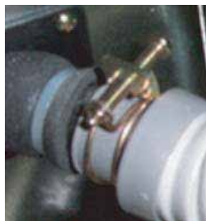
Clamp the Flexible Drain Hose Connection
