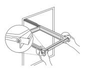
2 Keeping both levers pressed, lift the drawer support slightly and remove it from the rail system.
