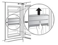
2 To lower the EasyLift bin, press up to release the levers at the bottom of the bin and lower the bin until it clicks into place.
