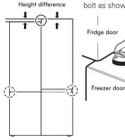
Adjusting Freezer Door Height Open the freezer door and use a wrench to rotate the door hinge bolt as shown.
