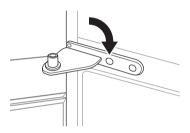
5 Tighten the two hinge bolts.
