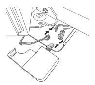
3 Position the bottom hinge cover in its place1 and tighten the cover screw 2.
