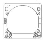
e. Remove the three screws on the hinge at the bottom left. Remove the hinge and reinstall it on the right side. The top screw will occupy the hole where you removed the screw behind the hinge bracket in step d.
