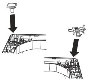
f. Insert and tighten the screw connecting the upper hinge assembly to the top lock rod, removed in step a.
