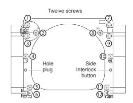
**5** Switch the door strike and the blank cover. Remove the two screws on the door cover that secure the door strike.
