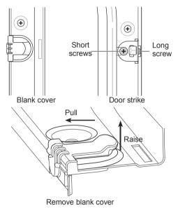
Gently pry out the hole plug on the side of the door cover and install it in the hole on the opposite side.
