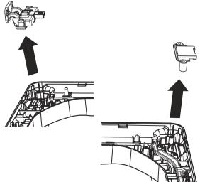
c. Lift out the upper hinge assembly (on the left).
