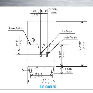
. Separate ICE and WATER Dispensing • LED Remote Sensor for hands-free operation
