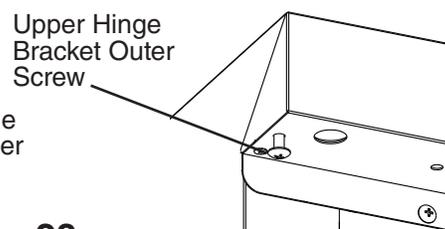
17) Be sure the lower hinge bracket thrust washer is in place, then place the door on the lower hinge bracket in the fully open position. Slide the door upper hinge bracket outer slot onto the upper hinge bracket outer screw. See Fig. 29.
