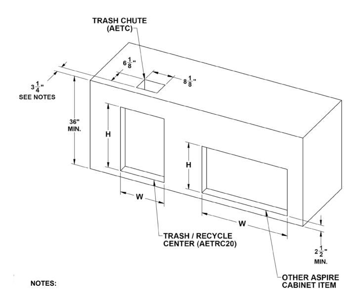
3-1/4" DIMENSION FOR TRASH CHUTE IS MEASURED FROM FACE OF ISLAND STRUCTURE AND DOES NOT INCLUDE ANY OVERHANG FROM A COUNTERTOP.
