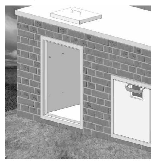
4. Reinstall the drawer(s) by aligning the slides on either side and pushing the drawer back into the opening. You will hear the release levers click. Open and close the drawer a few times to check for proper function and alignment. There are adjustment screws on either side of the drawer should vertical adjustment be needed.
