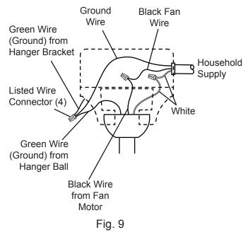
**NOTE:** Diagram shows wiring for single control of fan
