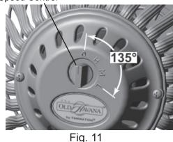
**NOTE:** If using the Wall Control (CH1) or the Remote Control (CH4), the 4-position fan speed control MUST be set on HIGH.
