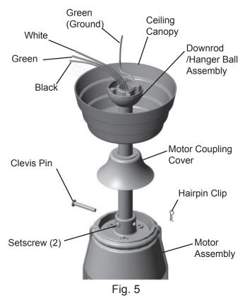
16. The fan comes with green, black, and white leads. Before installing fan, measure up approximately 6-9 inches above top of Downrod/Hanger Ball Assembly. Cut off excess wire and strip back insulation  $\frac{1}{2}$ " from end of wire.
