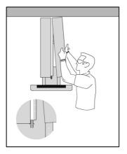
Place lower duct covers using one plastic bracket at each vertex (4 needed).
