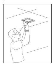
· Fix the upper horizontal support with 4 wood screws.
