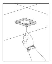
Attach the vertical supports (inf) (A) to the hood.
