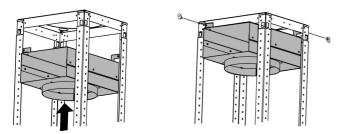
Measure from the bottom of the air deflector to the bottom of the hood outlet, as shown.
