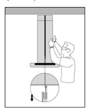
The lower duct cover shall be secured to rangehood by 4 screws.
