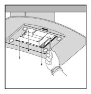
Install the grease filter and turn power on at service panel. Check operation of the hood.
