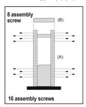
Attach a second vertical support set to adjust the vertical distance.
