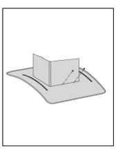
Attach the assembly to the support fixed on the ceiling. Assure with screws (16).
