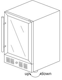
**Note:** Once you are ready to install the unit in a cabinet or directly on the floor, you must adjust the feet to level the refrigerator.
