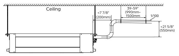
5. If connecting multiple drain pipes, install the pipes as illustrated below.
