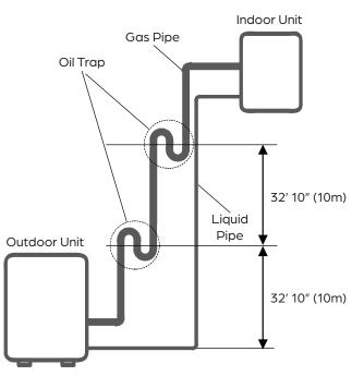
Required distance between oil traps when the indoor unit is installed higher than the outdoor unit.
