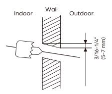
3. Place the protective wall hole sleeve (field supplied) into the hole. This protects pipes and cables from sharp edges and will help seal the opening when you finish the installation process. After the sleeve is inserted through the wall, connect the wall hole sleeve cover to the wall sleeve on the outside end. Make sure the cover is flush with the outside wall.
