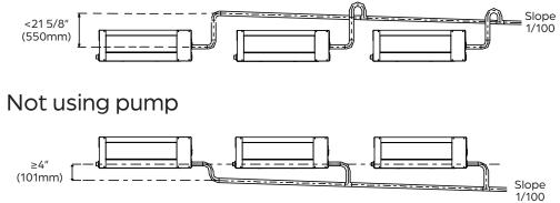
6. Pass the drain pipe through the wall hole to the outside. The end of the pipe should be at least 2" (50mm) above the ground. If it touches the ground, the pipe may become blocked. Make sure the water drains to a safe location where it will not cause water damage or a slipping hazard.
