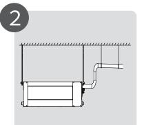
Install the drain pipe
