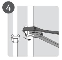
Connect the refrigerant pipes
