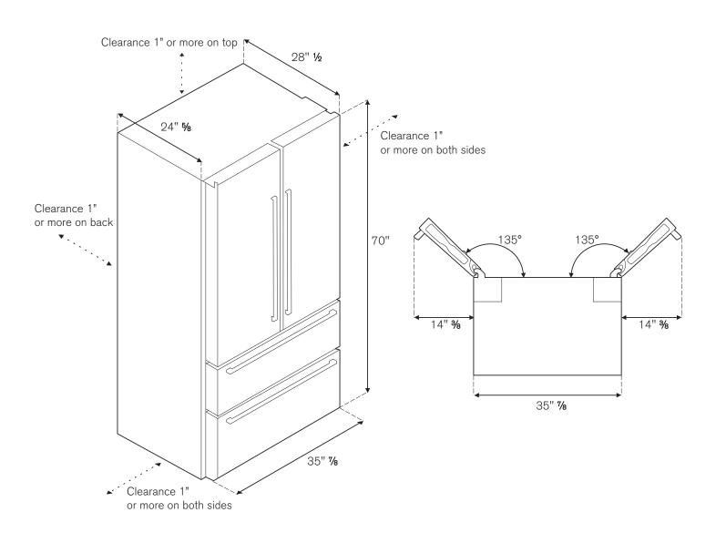
INSTALLATION: There shall be a space not less than 1 inch from the top of your refrigerator and not less than 1 inch from both sides or the back of the refrigerartor to the adjacent walls respectively. This requirements is good for open and close of the door and also for heat emission.
