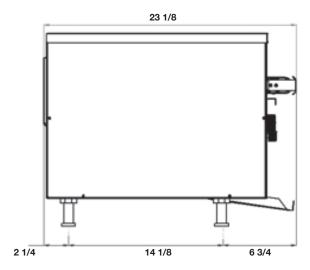
**INSTALLATION:** Counter model; furnished with 2 1/2" adjustable legs and 4 foot cord. Units should be located so that the air around the fan motor intake under the toaster, does not contain grease or steam and does not exceed 100°F.
