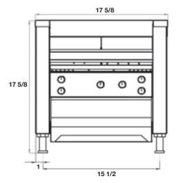
**CONTROLS:** Each chamber features Separate, Top, Variable Heat Controls; Variable Conveyor Speed Control; <u>Power Saver Switch</u>; and a Common High Temperature Limit Switch.
