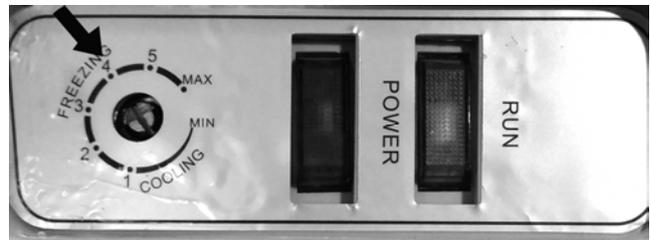
Setting the temperature control to the coldest setting may cause the evaporator coil to freeze and ice up. This will eventually result in a warmer cabinet temperature.
