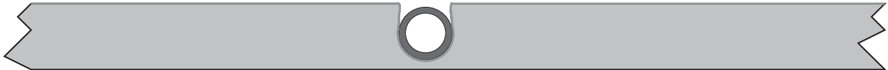
Figure A-1 A cross section, showing Zurn PEX pipe in groove and panel with aluminum top layer.
