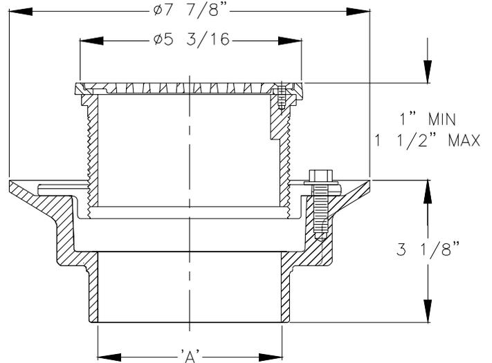
**FD-2290-ST Adjustable Finished Area Floor Drain with Square Top**
