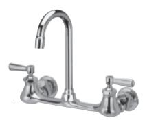
Polished chrome-plated cast brass 8" [203mm] sink faucet with quarter turn ceramic disc cartridges, 3/8" [10mm] short swivel inlets providing adjustable centers from 7-1/4" [184mm] to 8-3/4" [222mm] and a 3-1/2" [89mm] centerline rigid or swing gooseneck spout with a 2.2 GPM [8.3 L] pressure compensating aerator (complying with ANSI A112.18.1 Standard for flow). Unit is furnished with 2-1/2" [64mm] vandal-resistant color-coded metal lever handles.
