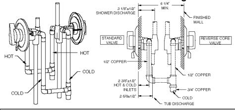
The ZURN TEMP-GARD Pressure Balancing Shower Valve is equipped with an adjustable limit stop screw. The limit stop device is to be used to limit the valve handle from being turned to undesired hot water discharge temperatures. To adjust the limit stop screw, remove handle and escutcheon, turn valve to maximum desired temperature and turn the limit stop screw until it seats. **IMPORTANT: Failure to adjust the limit stop screw properly increases the chances for serious injury.**
