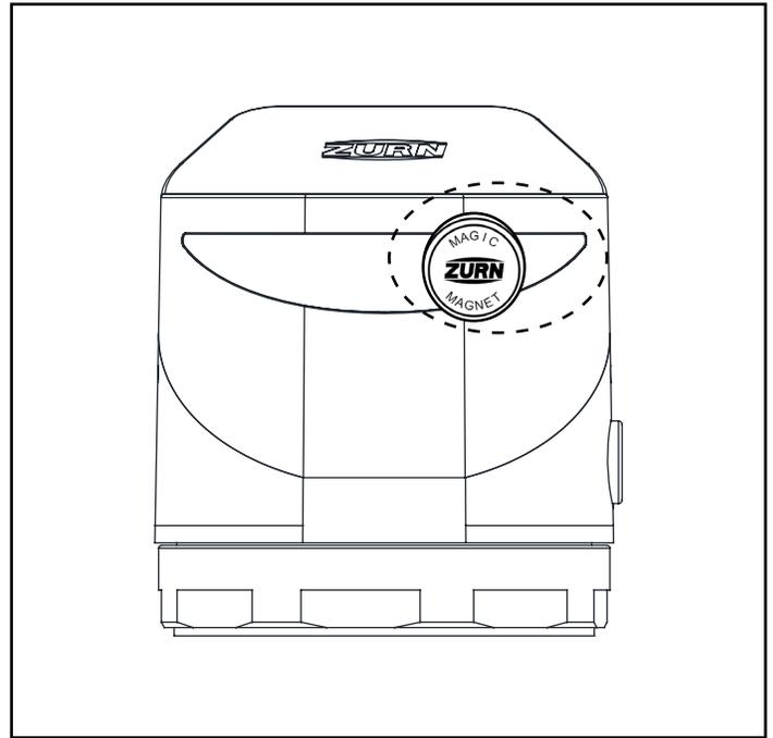
Note: To ensure proper functionality, make sure the calibration distance in water closet applications prevents the sensor from detecting the stall door. Verify this by closing the door for 10 seconds, then opening it. If the flush valve doesn't activate, the calibration distance is suitable. Otherwise, recalibrate to a closer distance using the magnet.
