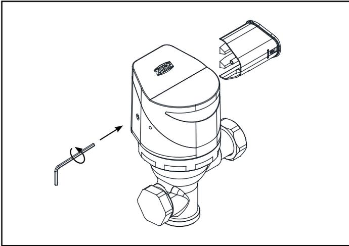
2. As shown, insert 6 (for battery-powered) or 4 (for hardwired) AA Alkaline batteries (supplied) into the battery tray.
