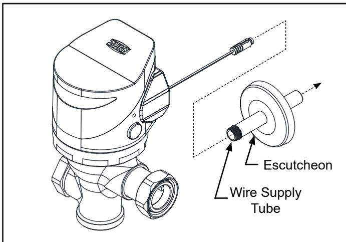
2. Insert both the power supply cable and wire supply tube into a thru-hole on the wall. Hand-tighten the wire supply tube into the battery tray and secure the escutcheon with the set screw.
