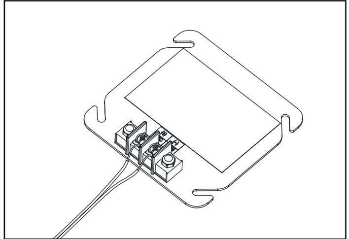
Optional -MJ Junction Box (Recommended when three or more flush valves utilize one HW6)
