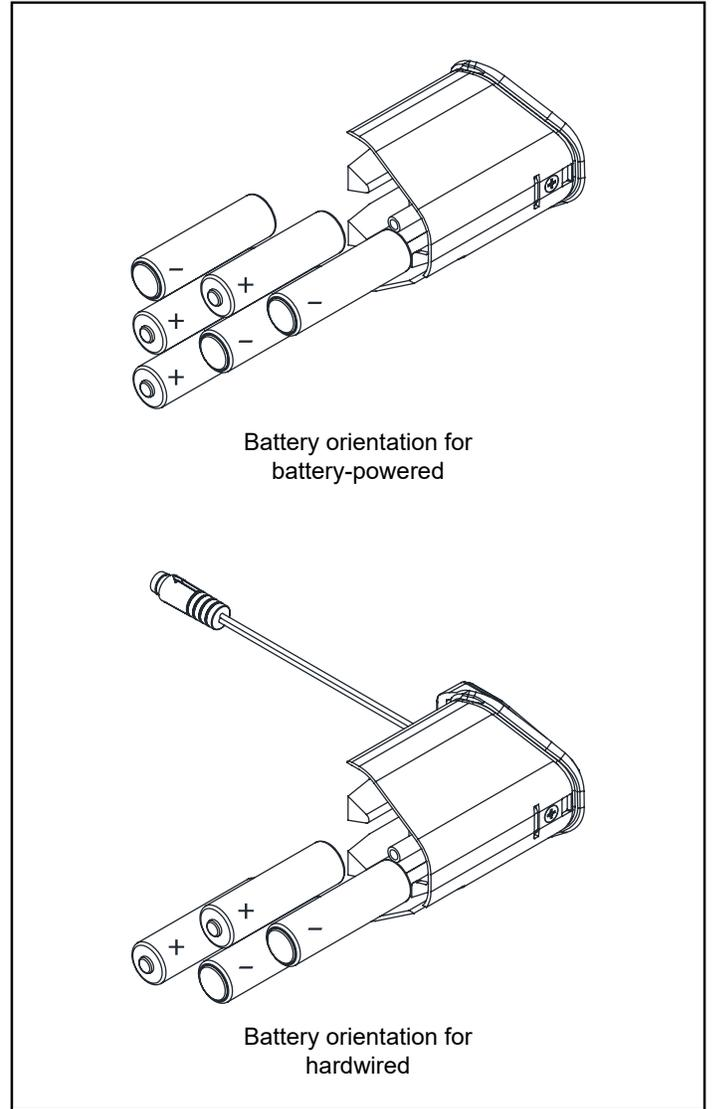
3. Slide the battery tray back into the valve head and apply firm pressure. Turn the 3/32" Allen Wrench clockwise to tighten the battery tray screw to a dead-stop and ensure the battery tray is flush with the valve head.
