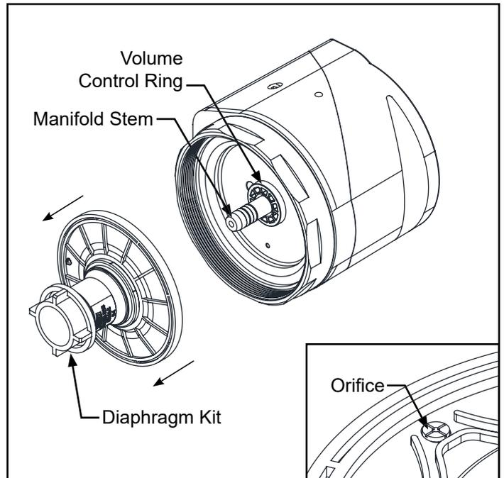
4. Place the valve head with the diaphragm kit back onto the valve body. Ensure that both the strap wrench and locking ring are dry for a better grip. Tighten the locking ring to its original position using the supplied strap wrench by turning it clockwise.
