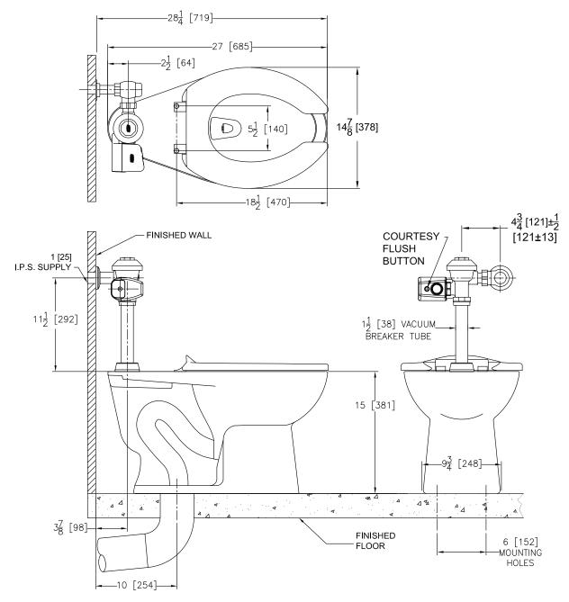
This system complies with the Buy American Act: Fixture manufactured in China; Valve manufactured in US with US and foreign parts. Meets the American Disabilities Guidelines and ANSI A117.1 requirements when installed according to these requirements. Fixture - Complies with ASME A119.2 / CSA B45.1 Faucet - Complies with ASME A112.18.1 / CSA B125.1
