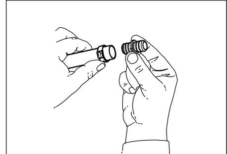
3. Push fitting into the tubing until the shoulder of the fitting is against the end of the tubing.
