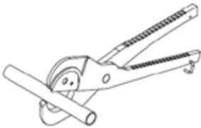
A wheel type of cutter works well for copper tube.
