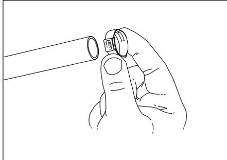
2. Slide the stainless steel clamp onto the tubing.
