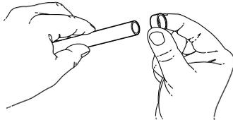
3. Now insert the fitting into the tube up to the fitting shoulder. Position the crimp ring 1/8 inch to 1/4 inch from the end of the tube. An improperly positioned ring may produce a weak connection. Ring may be squeezed to hold it in place until step 4 is completed.
