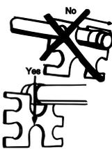
Do not slide the gauge onto the connection. Push it directly onto the crimp ring.
