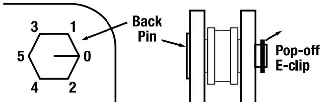
For a tighter crimp, turn mark on pin to the next number:
