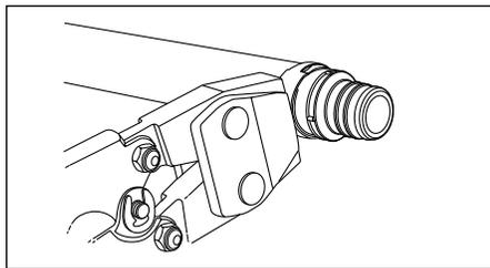
5. Position the open tool over the stainless steel clamp ear at a 90° angle. Completely compress the tool handles to close the tool over the clamp ear.
