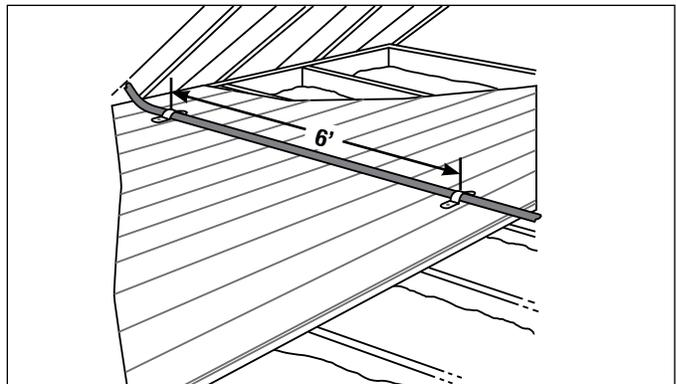
Straps can be as far as 6 feet apart if the pipe is continuously supported.
