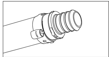
6. Remove the tool. **Note:** The crimp tool will not release until the connection has been made.
