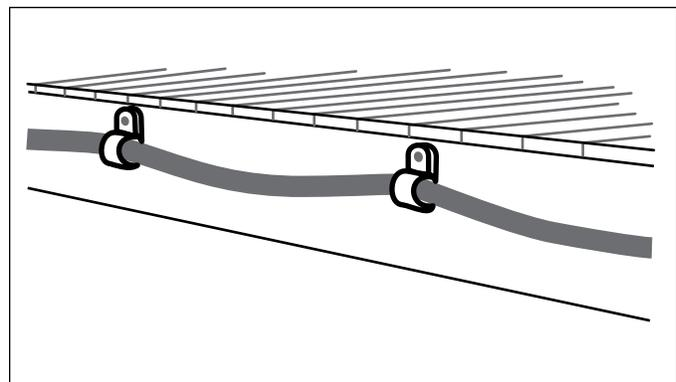
Always cut the pipe longer than necessary to allow some slack for any contraction in the pipe. 1/8" per foot of length is usually enough.
