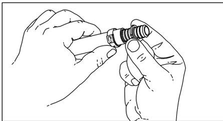
4. Position the stainless steel clamp so that it is 1/8" to 1/4" from the end of the tubing. **Important:** An improperly positioned ring may produce a weak condition.
