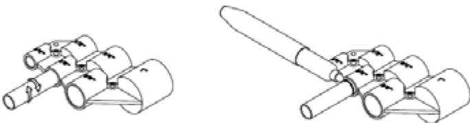
5. Insert the polybutylene tube into the polybutylene end of the Z-Bite fitting until it bottoms out in the fitting socket. Some resistance can be expected as the end of the tube moves past the teeth on the retaining ring and o-ring seal. The mark for insertion depth should be visible approximately 1/8" from the end of the fitting.
