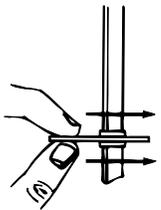
Always place the gauge opening on the crimp ring at a 90° angle for an accurate check.
