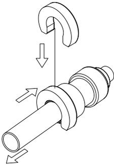
2. Place the appropriate sized Z-Bite removal clip on the tube with the grooved side facing the fitting.
