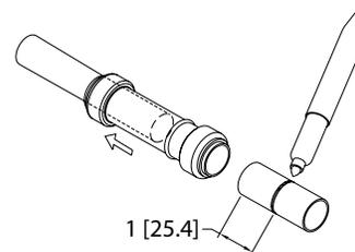
3. Deflect one of the tubes and slide the long end of the slip coupling into place until it hits the tube stop.
