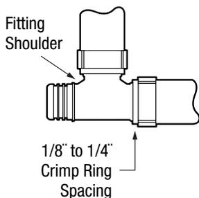
4. Position the tool so the crimp ring is completely covered by the tool jaws. Keep the tool at a 90° angle to the fitting and close it completely. Squeeze handles together to complete the crimp.
