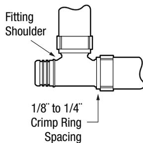
4. Position jaws squarely around the ring. Release upper handle to close jaws on the ring. Squeeze handles together to complete the crimp.
