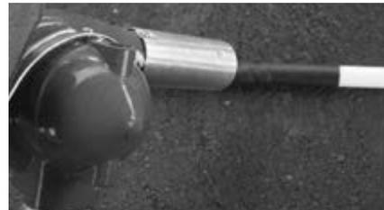
2. The heat shrink must be applied using a hot air gun. Do Not Use Open Flames or a Torch.
