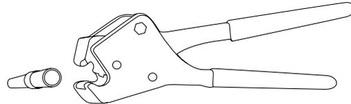
5. Pull back on moving handle to release jaws from crimped ring.
