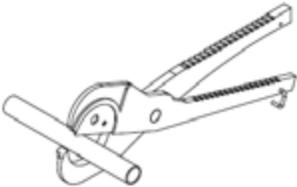
2. Using a blade-type tube cutter, cut the end of the polybutylene tube square.
