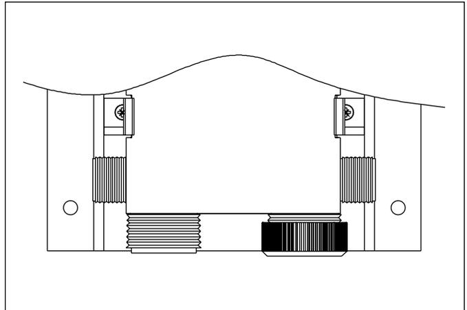
The 1" outlets can be fitted with a crimp x swivel or nut-ring-cone connector. These can then be used to supply high flow rate fixtures such as whirlpool baths, hose bibbs, etc. The unused 1" outlets need to be sealed using a 1" brass cap (Part No. QTC5FBG).
