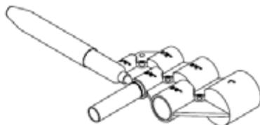
4. Examine the fitting to be sure that the tube liner is present. This liner is required when using PEX tube. If using copper or CPVC tube, the liner may be removed. See Tube Liner Removal instructions.
