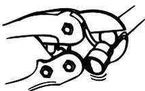
Do not try to save time by re-crimping a crimp that does not gauge properly. The fitting must be cut out and replaced.
