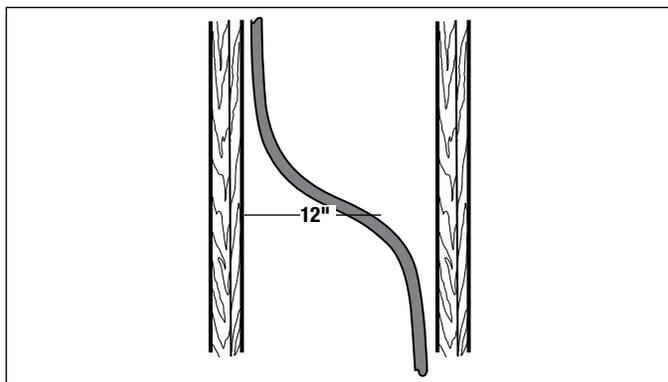
Since Zurn PEX tubing expands or contracts one inch for every 100 feet of pipe for every 10° of temperature change, you must allow for expansion and contraction in long runs with a 12-inch horizontal offset.
