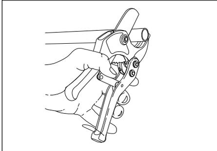
1. Measure and cut the tubing. Be sure you have a square, burr-free cut. An uneven or jagged cut may cause an improper connection.
