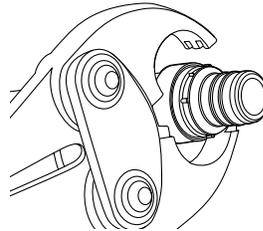
5. Open the tool handles to release jaws from the crimped fitting.
