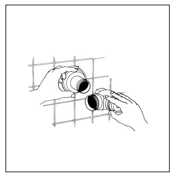
**1** Install stop valve using proper supply escutcheon and sweat solder kit if applicable.
