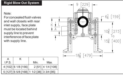
Lay out all necessary closet fittings on floor. To obtain spacing between units, place proper lengths of pipe between adjoining fittings (or use ZE-Series).
