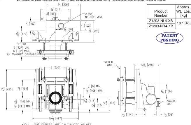
\* PULL-OUT FORCES ARE CALCULATED VALUES, WITH STANDARD COUPLING ASSEMBLY. NO SAFETY FACTOR HAS BEEN APPLIED.
