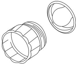
To replace the two G9 halogen light bulbs located at the upper left and right corners of the oven, unscrew the protection cap that projects out inside the oven.
