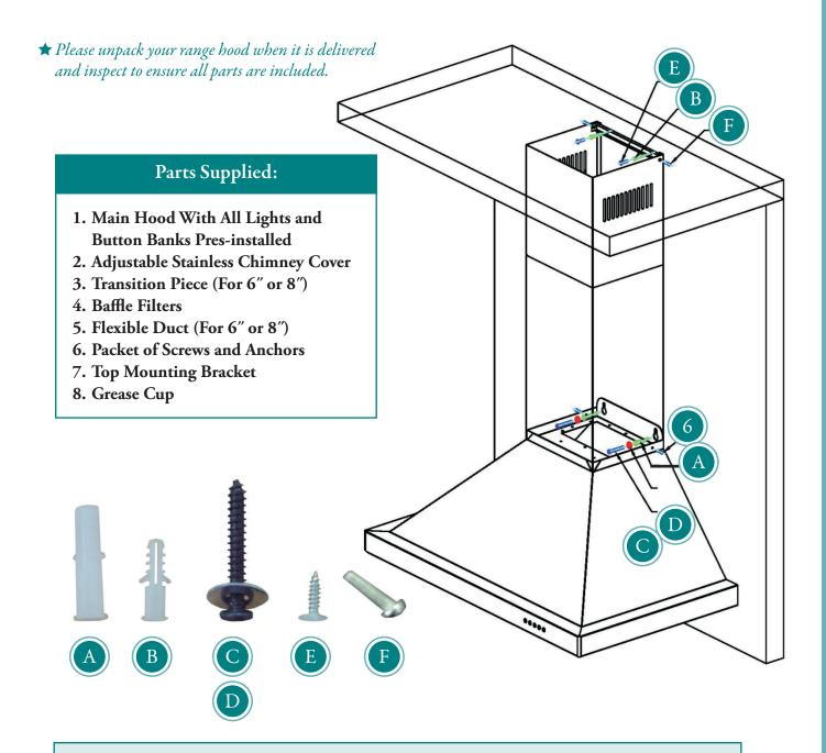
\*Note: Wall range hoods with single motors will come with a square to 6" round transition piece and will include a back draft damper. The ducting with these range hoods is 6".
