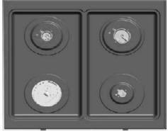
Dual Burner LPG: 1.27 - L20 NG: 2.38 - N21 Auxillary Burner LPG: 0.65 - L6 NG: 1.04 - N6
