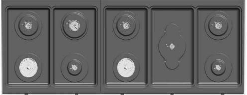
Dual Burner LPG: 1.08 - L15 NG: 1.79 - N15 Auxillary Burner LPG: 0.65 - L6 NG: 1.04 - N6 Dual Burner LPG: 1.08 - L15 NG: 1.79 - N15 Fish Burner LPG: 0.90 - L10 NG: 1.45 - N10 Auxillary Burner LPG: 0.65 - L6 NG: 1.04 - N6
