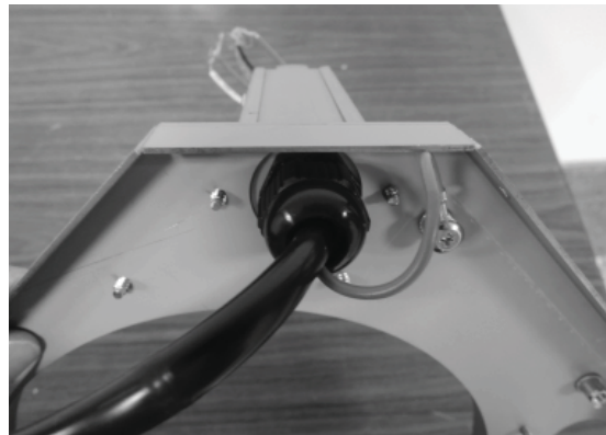
4. Secure ground wire to underside of internal blower flange by (1) 3/16*3/8 screw and (1) washer.
