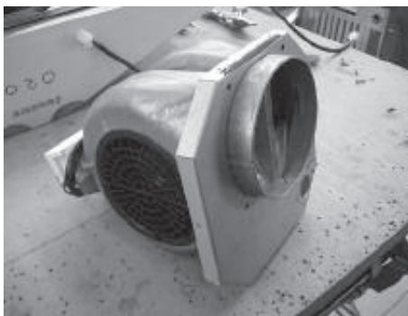
4. Position internal flange over blower housing.
