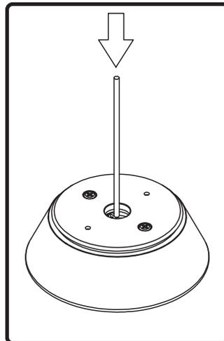
2. Place a pen or screwdriver in the bottom opening to dislodge the top touch panel.
