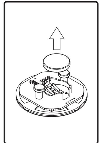
4. Install (1) CR2032 battery and reassemble the remote body.
