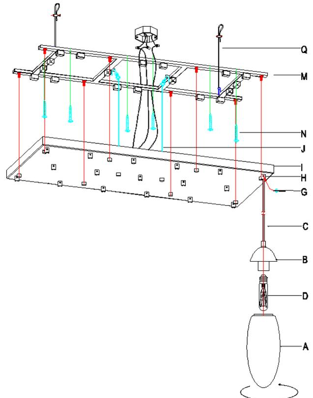
In Instruction: This fixture is provided with a Safety Cable. The Safety Cable provides a back up system the mounting frame and the installation hardware. It is essential that the Safety Cable be properly installed. The Cable must be secured to a STRUCTURAL MEMBER of the building, and not to the outlet box. The Cable must be terminated with Steel cable lock kit specifically sized for the Cable per the following steps:
