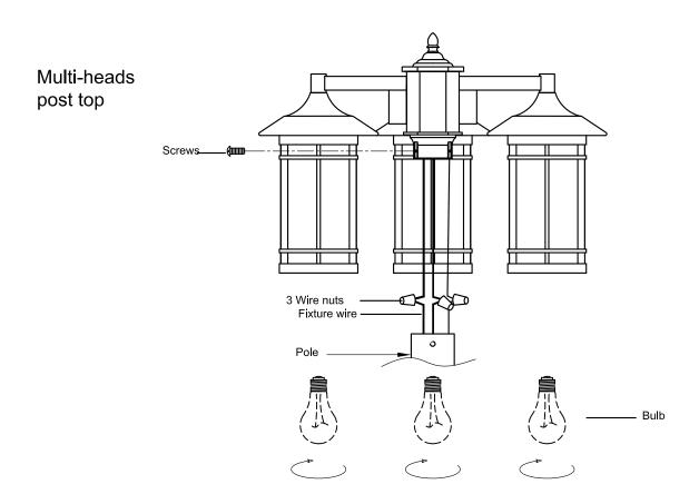
Please observe local building/electrical codes regarding the installation of your post fixture. Please keep in mind your geographic location and the depth that the ground freezes to, when deciding the depth of your installation. Column Hex screw (3) Post Base Cap Nuts (3) Spring washer (3) Anchor Bolts (3) Hex Nuts (3)
