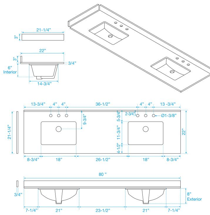
Note: Side splash is reversible. Due to high probability of breakage, the backsplash comes in two pieces, cut from the same piece. All measurements are  $\pm$  1/4".
