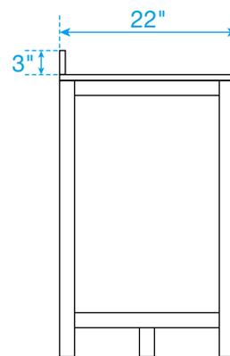
\*Note: Due to high probability of breakage, the backsplash comes in two pieces, cut from the same piece. All measurements are  $\pm 1/4"$ .
