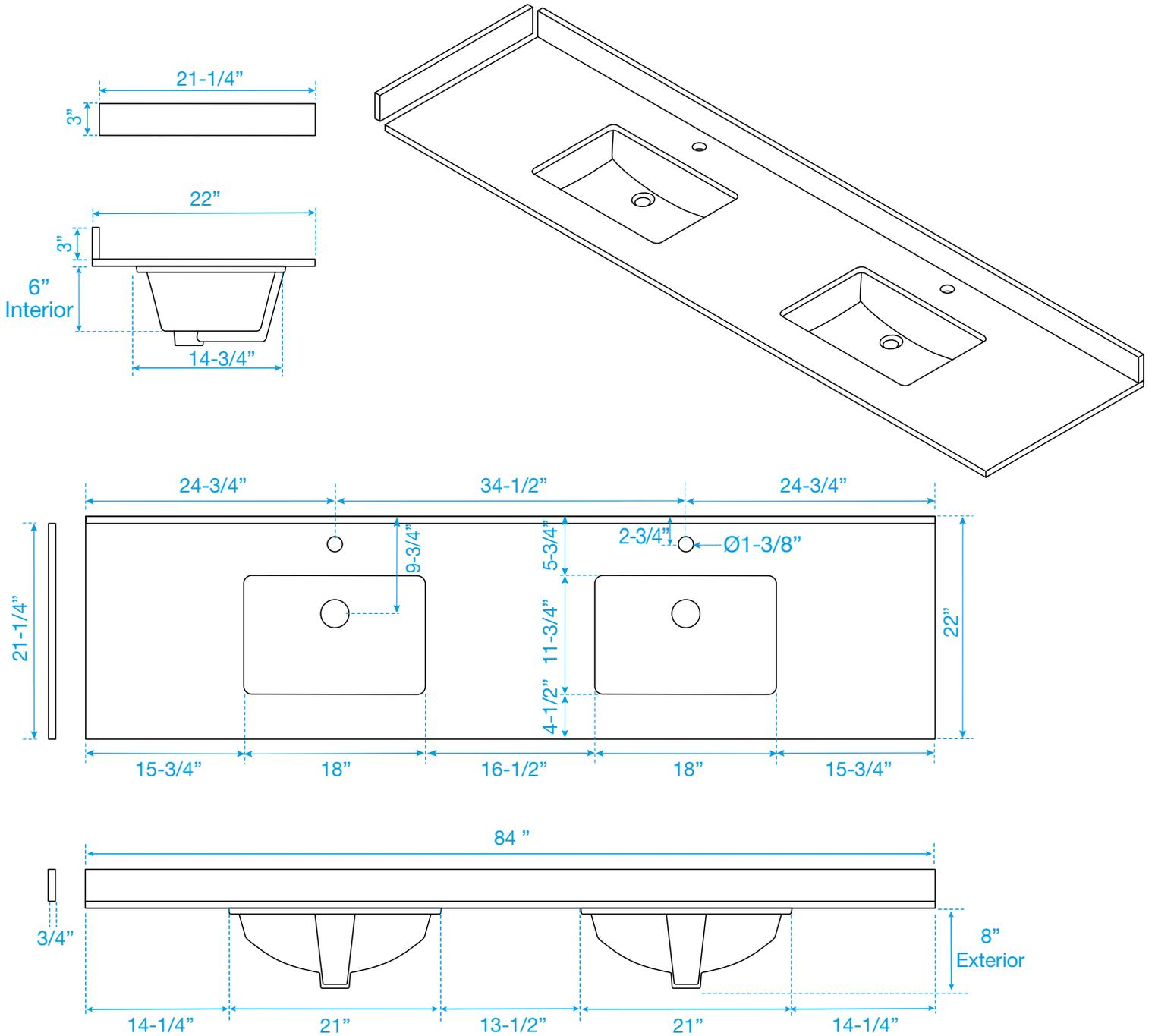
Note: Side splash is reversible. Due to high probability of breakage, the backsplash comes in two pieces, cut from the same piece. All measurements are  $\pm 1/4"$ .
