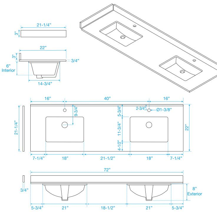
Note: Side splash is reversible. Due to high probability of breakage, the backsplash comes in two pieces, cut from the same piece. All measurements are  $\pm$  1/4".
