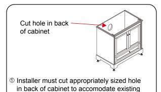
placement of hot & cold wall valves & drains.
