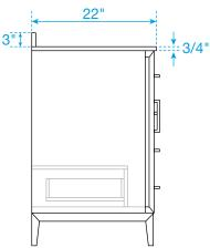
\*Note: Due to high probability of breakage, the backsplash comes in two pieces, cut from the same piece. All measurements are ± 1/4".
