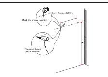
② Install the mirror: use a pencil to mark the placement of the screw holes on the wall, drill the holes and insert the plastic wall anchors.
