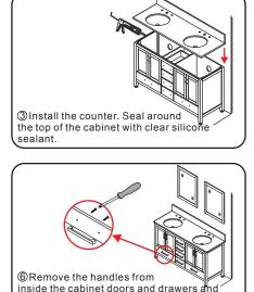
reinstall on the outside.Do not over-tighten
