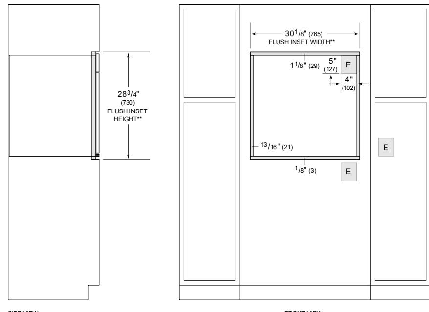
\*\*1" (25) minimum depth. Shaded areas will be visible and should be finished to match cabinetry.
