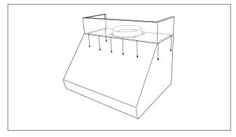
5 Six additional screws are provided to secure the top of the duct cover to an upper cabinet or soffit area, if accessible.
